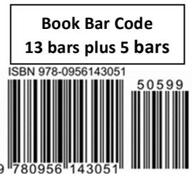
Not this time...the communication between the two suppliers failed to define the bar code accurately. The conveyor people ignored the second set of 5 bars, the software company programmed everything to use all 18 bars. As a result, the conveyor controls were built around 13 bars and the software was developed around 18 bars. It was a “simple” mistake.
